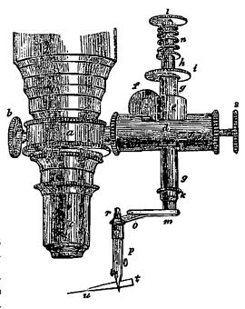
carries the small spring forceps p, which turns freely in the socket r. The forceps grasp the triangular slip of card t, which has a bit of human hair u, gummed to it, and projecting about  $r_0^1$  th of an inch.
